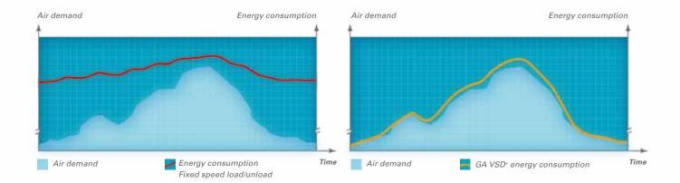
In almost every production environment, air demand fluctuates depending on different factors such as the time of the day, week or even month. Extensive measurements and studies of compressed air demand profiles show that many compressors have substantial variations in air demand.
